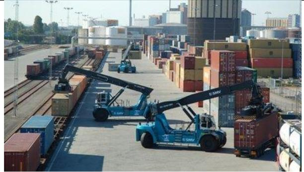
Figure 2: Intermodal handling using reach stackers
