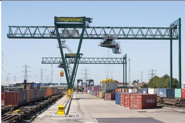
Figure 3: Intermodal handling using gantry cranes
