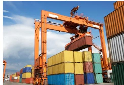
Figure 9: Rubber Tyred Gantry Crane (RTG)
